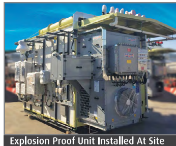
Explosion Proof Unit Installed At Site
